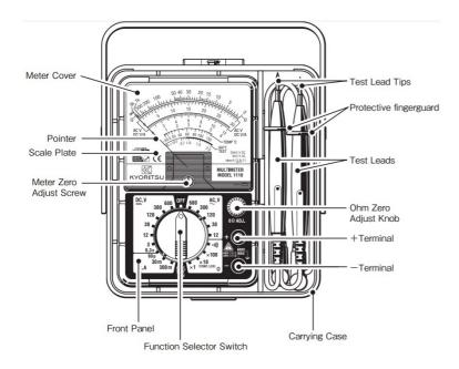
**Protective fingerguard:**It is a part providing protection against electrical shock and ensuring the minimum required air and creepage distances. Caution:Keep your fingers and hands behind the Protective fingerguard during measurement
