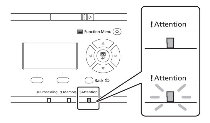
If an error occurs on the machine, the error message appears on the screen. Also the Attention indicator on the operation panel will light up or flash. Refer to the Operation Guide to Clear the error. For details, refer to the Operation Guide on the Product Library disc.
