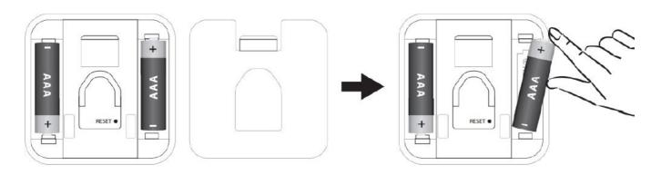
NOTE: LED will blink for 10 seconds to indicate low battery power. The estimated battery standby time is 8 to 12 months.
