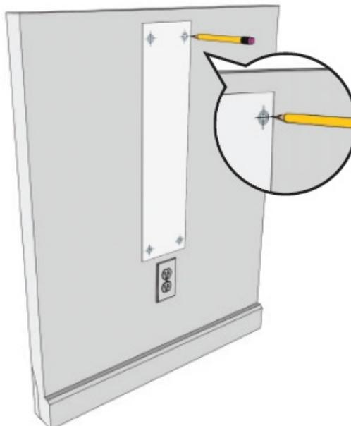
2. Using the markings created with the drilling template, drill 4 holes with a 3/16" drill bit. After drilling, insert a plastic wall anchor into each of the holes.
