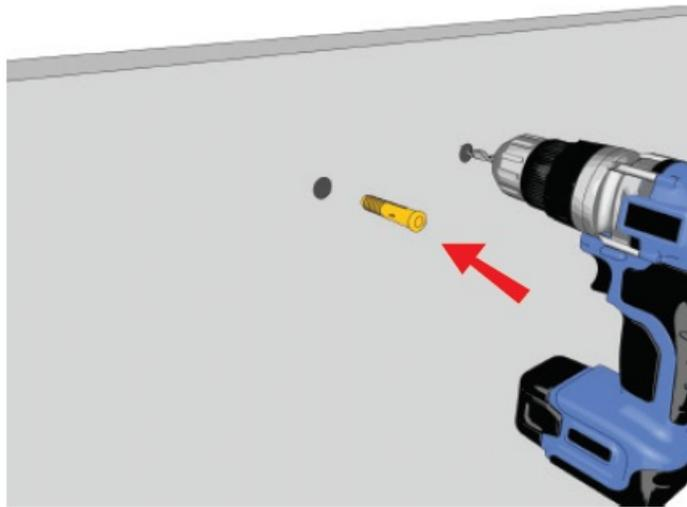
3. Drive mounting screws into the top two wall anchors. Do not drive them until they are flush against the wall. Leave a gap of approximately 1/8".
