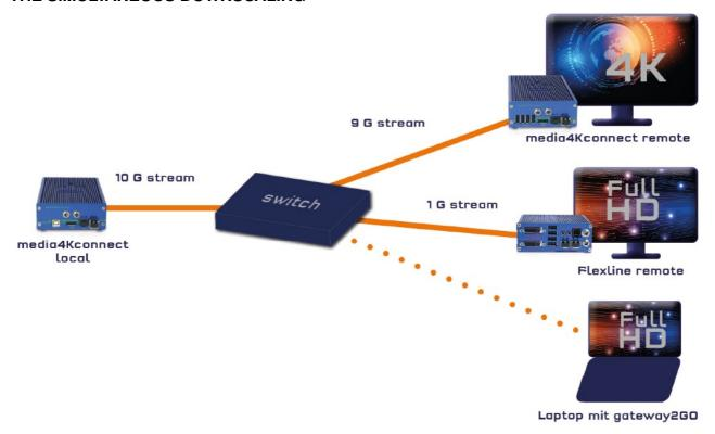
4K sources can be displayed simultaneously in 4K and with downscaling in Full HD on the remote unit. The output of the stream is done at 4K over 10G bandwidth. Two streams are transmitted simultaneously, so the 4K stream has 9 GBIT and the second stream in Full HD 1 Gbit. The streams can be routed and shared independently and one source can be split to any number of screens. One user has full USB control (keyboard and mouse etc).
