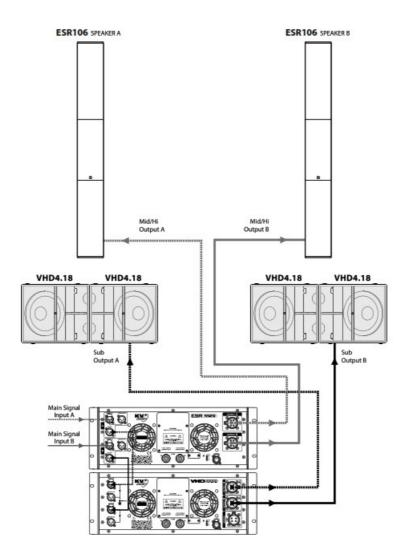
Set ESR2600D Amplifier to FULL RANGE OFF mode. Signal is crossed over at Hi/Mid for ESR106 cabinets and SUB for external subwoofer.
