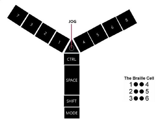
When you open the keyboard, there are four keys, left and right, and then the Jog Key is in the middle. The left and right keys are the same as the Braille arrangement. The key at the far left and right end is No. ② and No...
