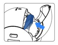
Press and hold the buttons on both 3 sides of the pedal at the same time, and put the pedal into the body.
