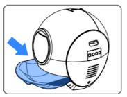
4 On the inside of the fuselage, Install the foam stopper.
