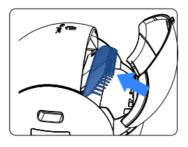
Remove the inner compartment cover.
