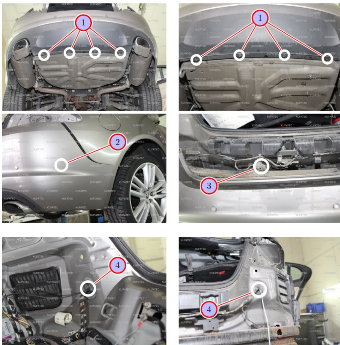
Figure 9: Disassembly bumper and cable routing
