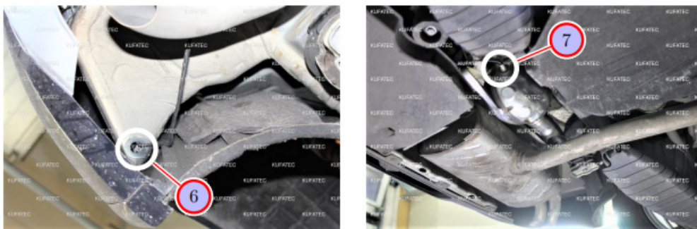
Figure 10: Cable routing to the sound generator
