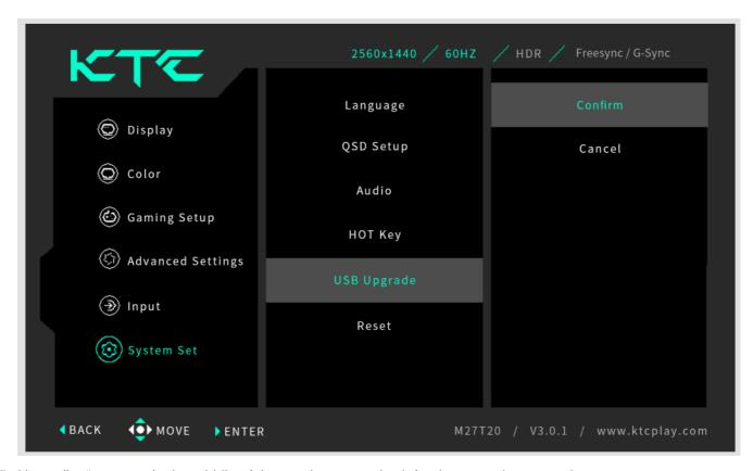
5. Upgrading" appears in the middle of the monitor screer; iwait for the upgrade to complete This process takes about 2-3 minutes, please do not cut off the power during this period; (There is a small probability that you will not enter the upgrade program after confirmation, you can repeat the third step).
