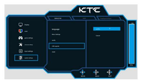
5. "Upgrading" appears in the middle of the display screen, and wait for the upgrade to complete (there is a small probability that the upgrade program does not enter after confirmation, you can repeat the third step)
