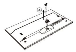
c. Undo the screw on the monitor;
