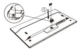
a. Install the base into the hole position and lock with two screws;
