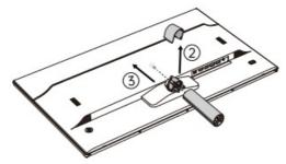
b. Undo the screw and open the cover on the base;
