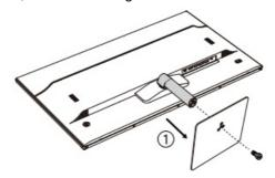
a. Undo the screw on the chassis;
