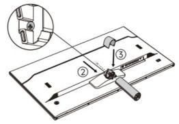
b. Lock the pillar with a screw and cover the back of the base;
