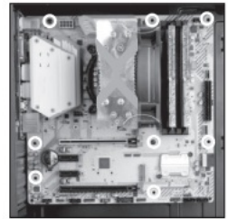
Screw motherboard using included screws.
