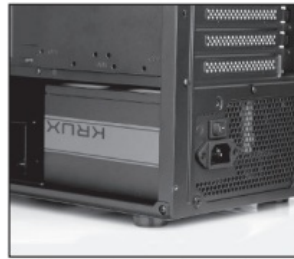
Insert PSU from the right side of the case.
