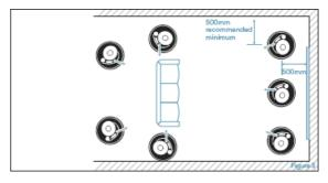
background music applications where the speakers must be placed near a side wall for aesthetic or structural reasons. In this application the IC52 can be used to project the sound towards the centre of the room.
