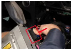
12. Plug the CarPlay 48PIN main line to the multimedia box.
