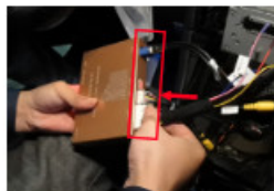
13. Connect the power cable (white one) to the carplay box, Connect the USB cable
