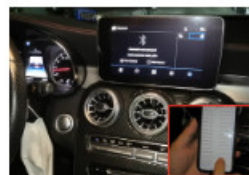
19. Keep phone WIFI ON, Open phone Bluetooth and searching (Find the Bluetooth name and pairing code of Smart box). Insert pairing code
