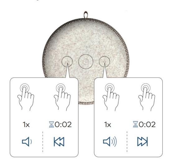
• Press the plus or minus button to adjust the volume. To skip tracks, press and hold the plus or minus button for 2 seconds.
