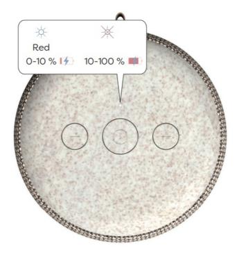
• The battery indicator is located on the top of the aCAPPELLA Wheat. The small light will turn red when the battery level drops below 10%
