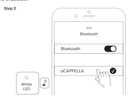
• Find aCAPPELLA Wheat in the Bluetooth list (in settings). When the light is blinking, the device is in Bluetooth pairing mode. The light will be solid white when connected to aCAPPELLA Wheat.
