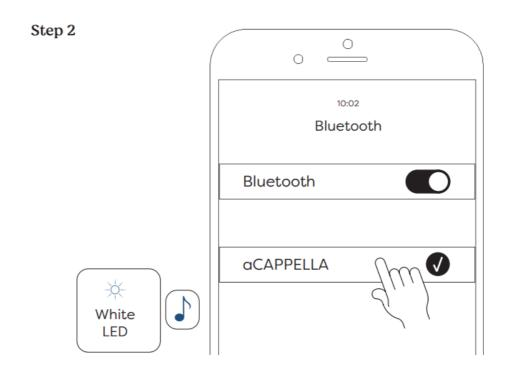
• Find a cappella Wheat in the Bluetooth list (in settings). When the light is blinking, the device is in Bluetooth pairing mode. The light will be solid white when connected to a CAPPELLA Wheat.
