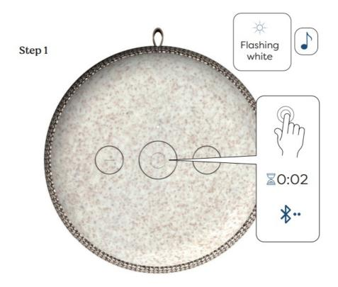
• To manually connect the aCAPPELLA Wheat to Bluetooth, press and hold the power button for 2 seconds. When the light blinks, the device is in Bluetooth pairing mode.
