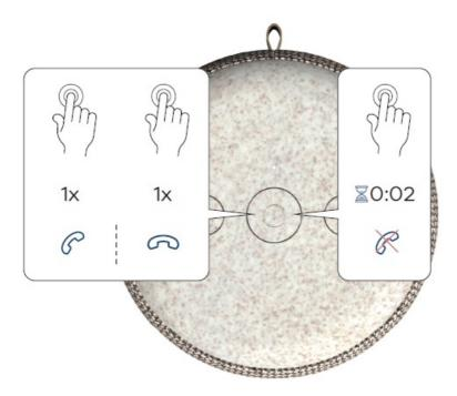
• Press the power button once to answer or end a call. Hold the power button down for 2 seconds to reject a call.
