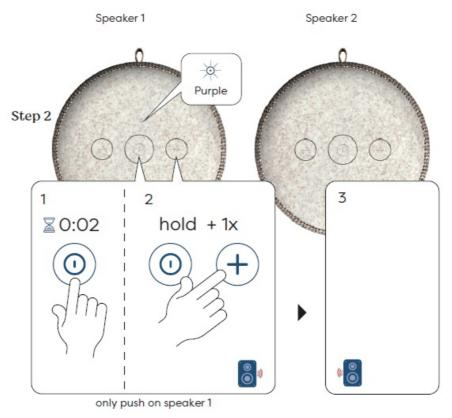
• Press and hold the power button until the speaker make a sound. Keep holding it, press the plus button once, then release both buttons. The small light will change
