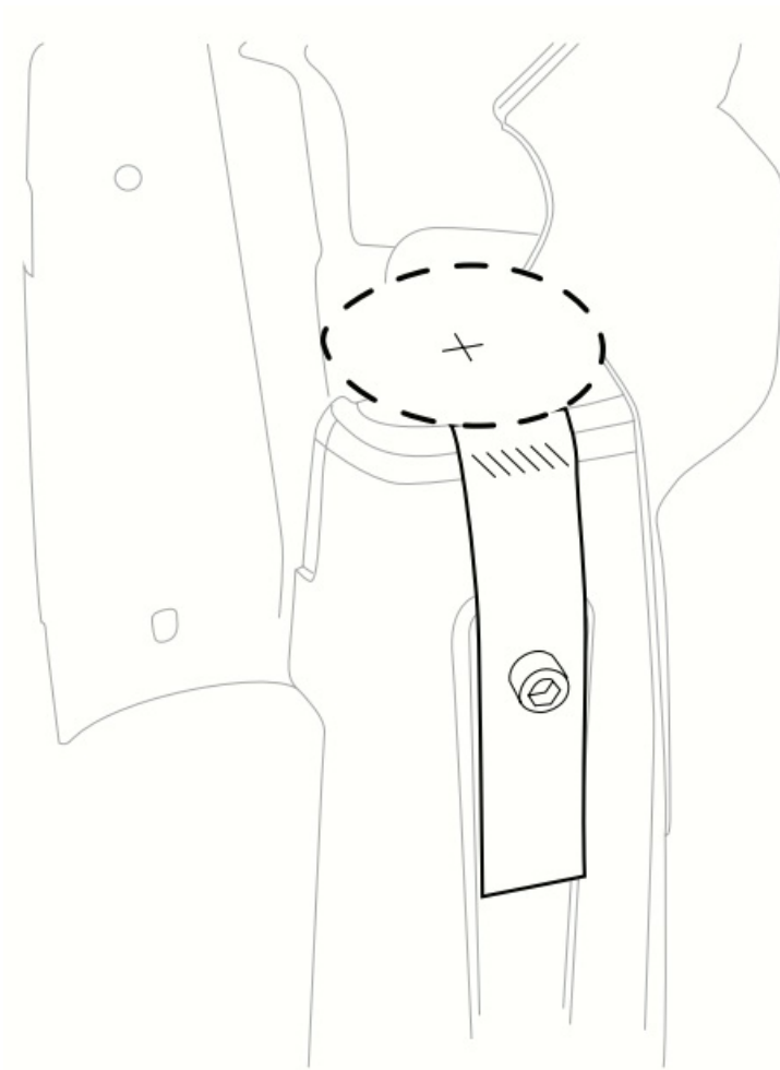
Road Glide Nacelle Fork Cap Clearance Cut Template Usage – Fig. B
