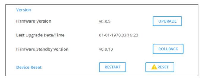
Figure 23: Device Settings Page – Firmware Upgrade
