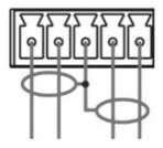
• Unbalanced Stereo Audio Input Connection
