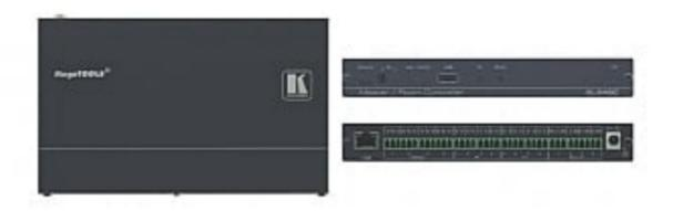
SL-240C is a compact master/space controller (Kramer Control brain) with PoE. It can operate over Ethernet with control interfaces that include: four bidirectional RS-232, four IR, four GPI/O, and four relays. It controls devices such as scalers, video displays, audio amplifiers, Blu-ray players, sensors, screens, shades, door locks, and lights. Multiple Kramer Ethernet control gateways can be used to add remote I/O ports
