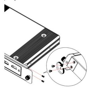
3. Attach the device to the panel using 4 screws (2 on each side to secure the device to the panel.
