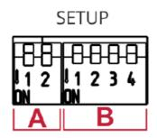
• The DIP-switches are used to set the HDBT range, upgrade the firmware, Determine IR signal pass-through.
