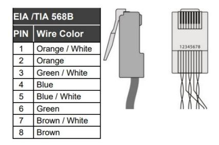
For HDBT cables, it is recommended that the cable ground shielding be connected/soldered to the connector shield.
