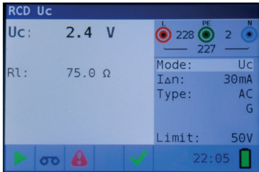
Figure 4 13: Example of contact voltage measurement results
