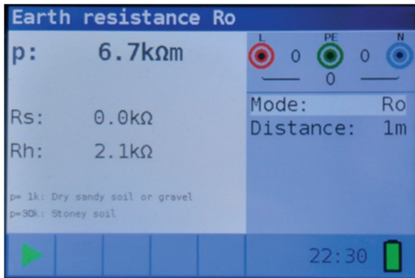
Figure 4 41: Example of specific earth resistance measurement results
