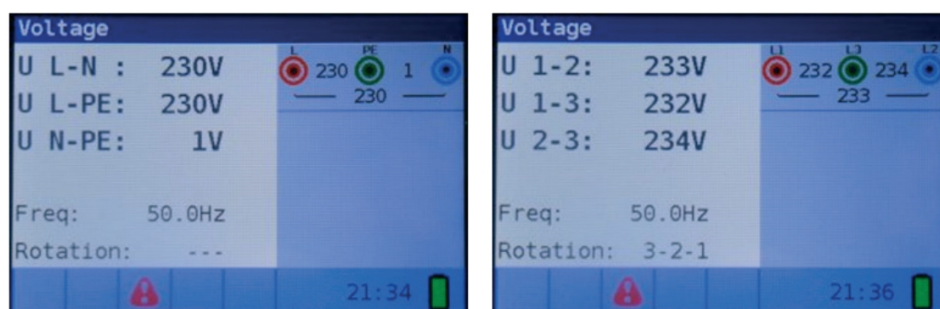
Figure 4 34: Examples of voltage and frequency measurements
