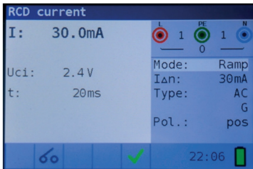
Figure 4 17: Example of trip-out current measurement result
