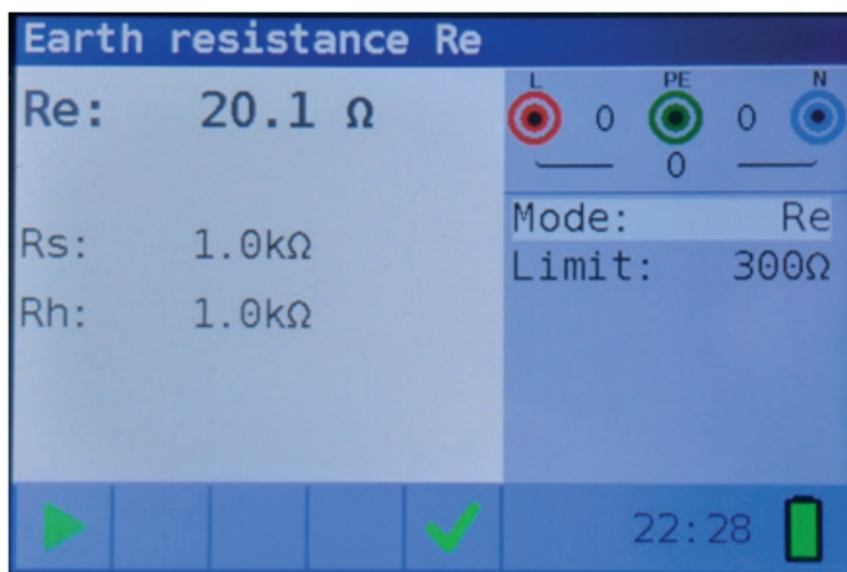
Figure 4 38: Example of resistance to earth measurement results
