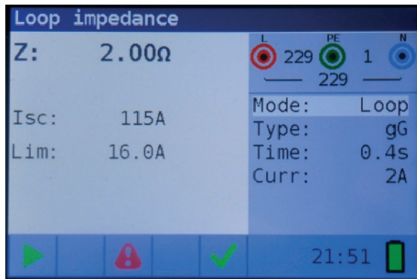
Figure 4 23: Example of loop impedance measurement results
