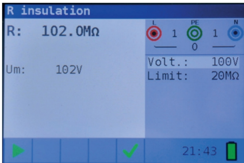
Figure 4 3: Example of insulation resistance measurement results
