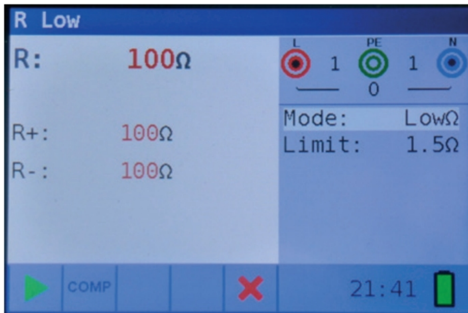
Figure 4 7: Examples of R Low resistance measurement results
