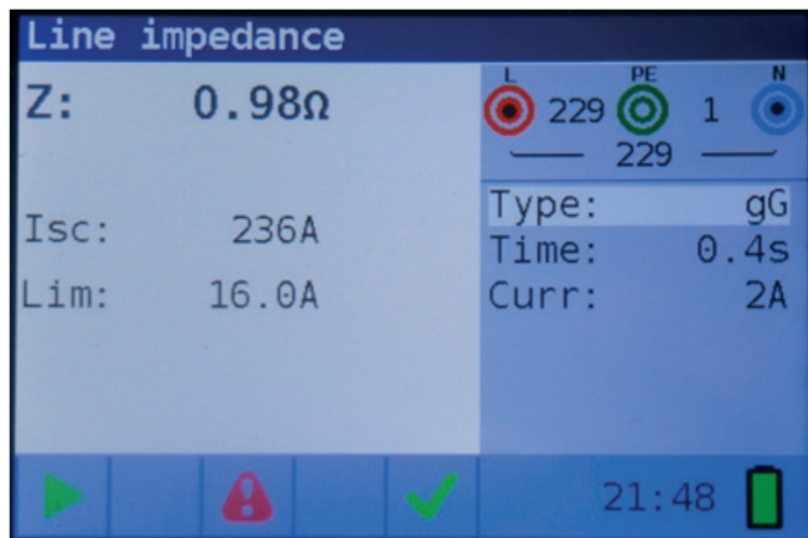
Figure 4-28: Example of line impedance measurement results
