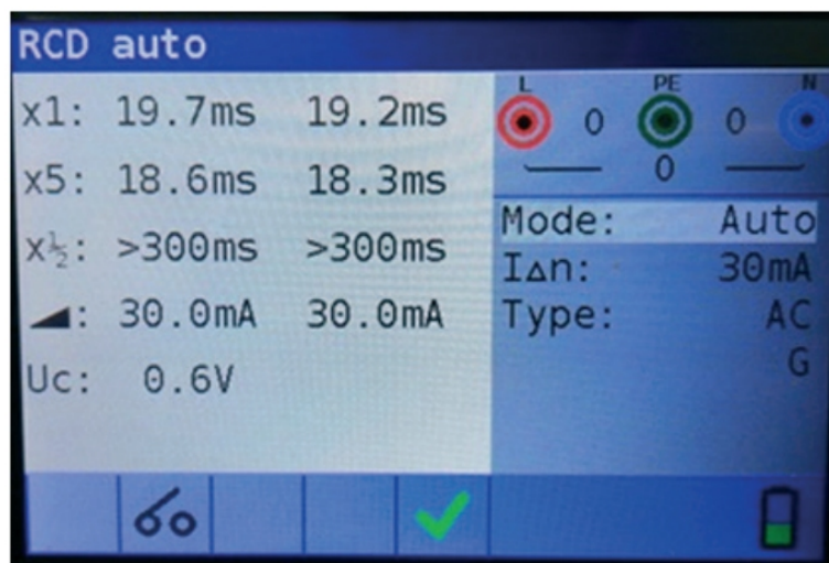
Figure 4 20: Step 8 RCD autotest results
