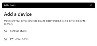
6. When "Connected" is shown, the pairing is completed, and you can use the Bluetooth MIDIconnection. Press [Done] .
