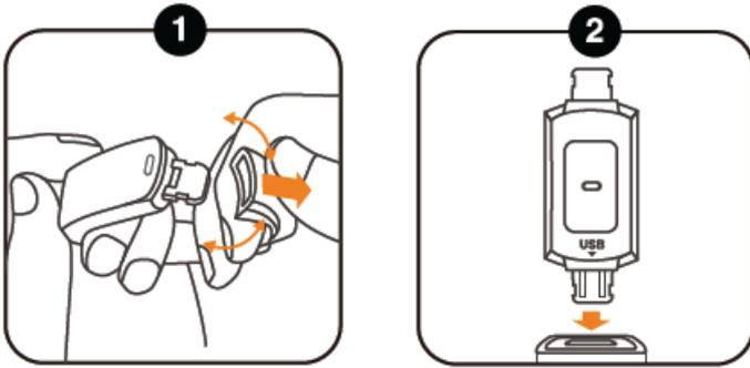
1. Remove the bottom wristband to access the charging connector with a twist and pull motion (refer to diagram 1 ). You can find the connector side under the KoreTrak marked “USB” with an arrow pointing at it, the USB metal contacts should be visible (refer to diagram 2).
