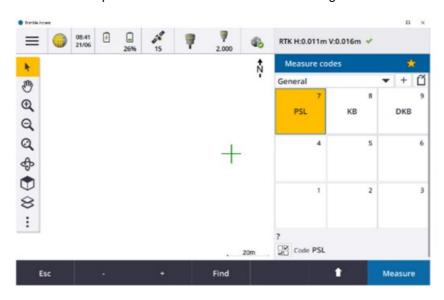
To measure a coded point, tap the button required. It is also possible to highlight a button by using the spider key on the TSC5/7 keypad and pressing the Enter button to take the measurement. String numbers can be attached to codes by highlighting the button required and using the – and + keys at the base of the screen.
