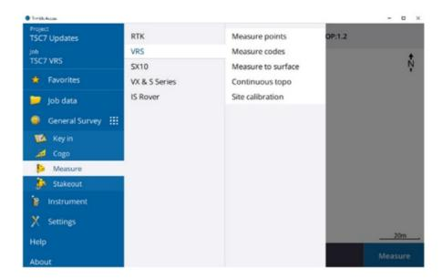
Access will use the Internet connection through the modem in the Controller to connect to the VRSNow data server.
