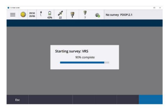
After a short period, initialisation will be gained giving you high precision values. Try to have the Receiver in an open area clear of obstructions whilst initialisation is taking place. The status bar at the top right corner of the Access screen will show the precision status with a green tick and the Horizontal and Vertical precisions.
