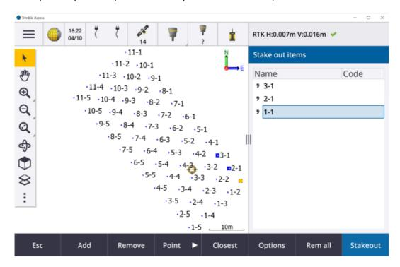
If more than one point is selected, then tap on the point in the list displayed to set it out, or tap the Closest button to set out the closest point to your current position. The Stakeout point screen will appear:
