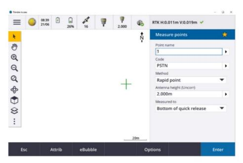
Points are measured by tapping the "Measure" button or pressing any of the Enter buttons on the Controller keypad. If Trimble Access isn't configured to automatically store measurements, then you will have to tap "Store" to save each point.
