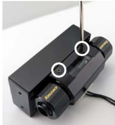
Secure with two screws on top
