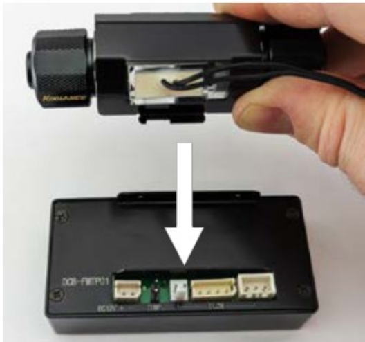
Hook the lower bracket tab into the display
