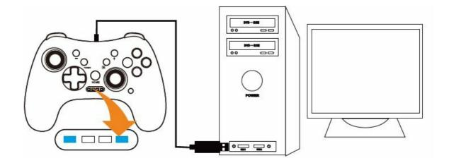
Under the mode of X-Input, press the HOME Dutton long to switch X-Input to DAnput Mode.
