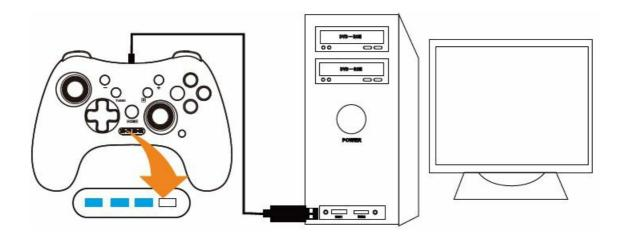
Connect controller to pc with type-c cable, after windows system recognized, the controller will start to work, LED 1,2,3 light will be long on.
