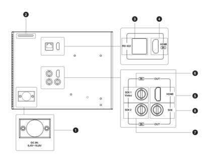
DC power input interface, power input range 8.4~16.8V.
