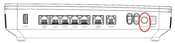
When you switch the home gateway on, pay attention to the light indicators. It takes about 90 seconds for the Innbox E94 home gateway to boot up; the POWER light indicators should be on uninterruptedly.
