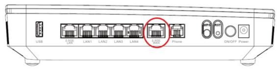
2. Plug the DC jack of the power-supply adapter to the POWER port on the device, and the other end to your electricity power outlet.
