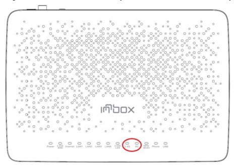
The transfer of the settings will be finished when 2.4G and 5G light indicators will be on interruptedly.
