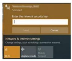
3. Use the Security Key printed on the label on the bottom part of the Home Gateway to connect to the Network.
