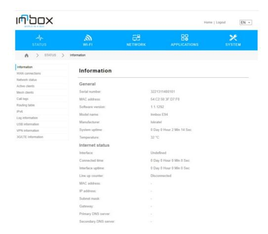
Top frame (navigation toolbar) lists main functions of home gateway Innbox E94. Left frame (navigation tree) lists the home gateway functions that you can change. The function names act as hyperlinks: when you click a link, the corresponding configuration page is displayed in the right frame. Right frame (display area) displays a configuration page for the selected function.
