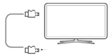
2. (**Optional**) If you have a set-top box, then connect one end of the HDMI cable to your Hub **I PUT** port and the other end to your HDMI connector on to your set-top box.
