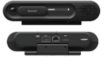
1. Connect one end of the HDMI cable to your Hub **To TV** port and the other end to the HDMI connector on to your TV set.
