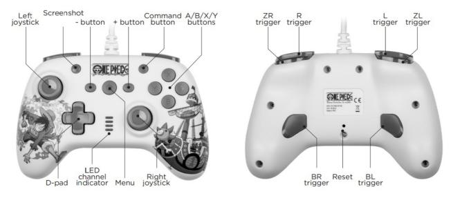
Note: Vertical press on the left joystick is L3; Vertical press on the right joystick is R3; Channel indicators are LED1, LED2, LED3, LED4 from top to bottom.
