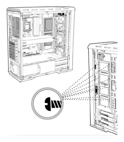
• Attach 2 screws to the left side of the hard drive. Slide the drive into the 3.5" bays at the rear of the case Secure the drive on the right side using the provided screws and hand tighten.
