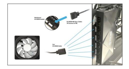
Connect up to 6 ARGB devices to the ARGB fan hub controller. 4 fans are pre-installed. Connect additional ARGB devices to the free headers. Connect the 5V ARGB MB sync. cable to the mainboard 5V ARGB header to control the lighting via the mainboard.
