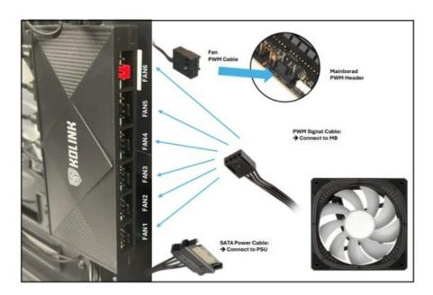
Connect up to 6 fans to the ARGB fan hub controller. 4 fans are pre-installed. Connect additional fans to the free PWM headers. Connect the PWM signal cable to a free mainboard PWM fan header (e.g. CHA\_FAN1) to control the fan speed via the mainboard. Connect the SATA power cable to a free SATA power connection on your PSU.
