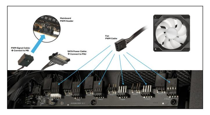
Connect up to 6 fans to the ARGB fan hub controller. 4 fans are pre-installed. Connect additional fans to the free PWM headers. Connect the PWM signal cable to a free mainboard PWM fan header (e.g. CHA\_FAN1) to control the fan speed via the mainboard. Connect the SATA power cable to a free SATA power connection on your PSU.
