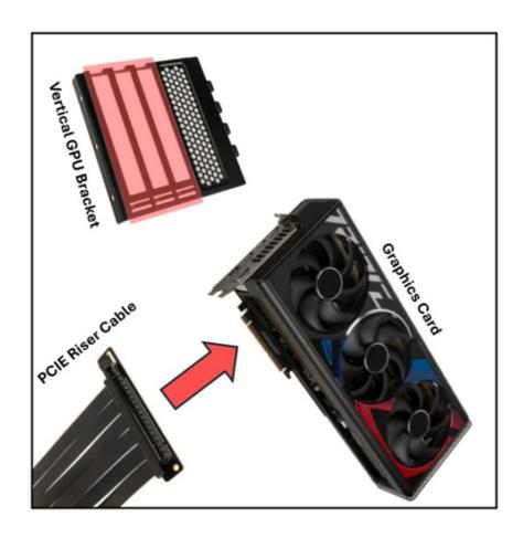
Mount the graphics card on the vertical GPU bracket in the preferred position.
