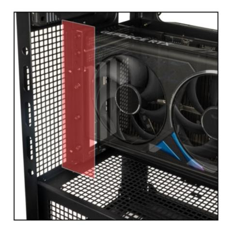
Mount the vertical GPU bracket with the graphics card attached to it onto the expansion slots.
