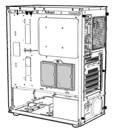
• Remove the bracket from the rear of the motherboard plate, attach your 2.5" drives and then screw back into place.
