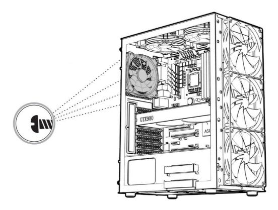
Align your fan to the screw holes on the chassis and secure with screws.
