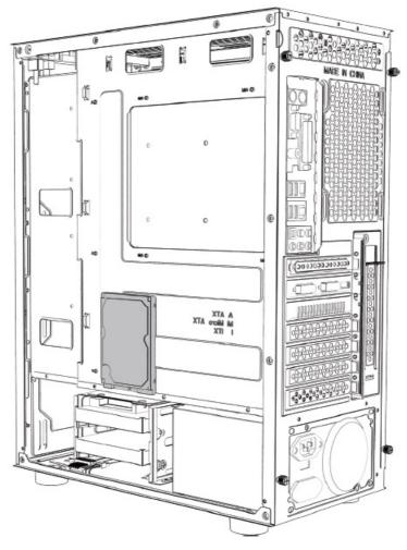
• Place the 2.5" HDD/SSD into/on top of the HDD bracket and screw in if required.
