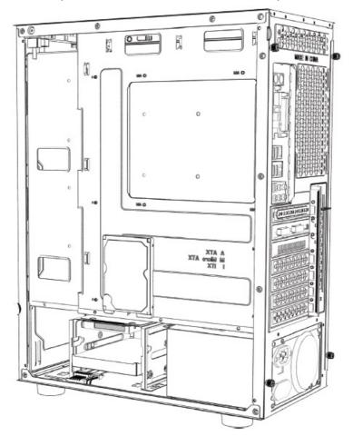
• Place the 3.5" HDD into/on top of the HDD bracket and screw in if required.
