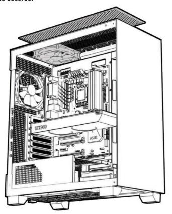
• Align your fan to the screw holes on the chassis and secure with screws.
