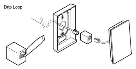
5. Hook the top of the interface onto the bracket, then press to click the bott om in place. To remove, use the tool to unlatch the bott om, then tilt out.
