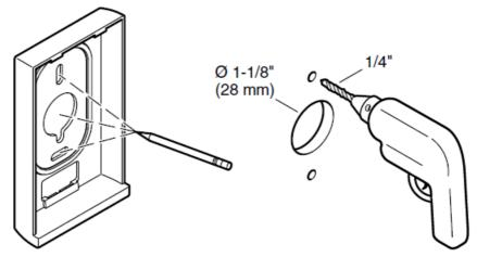
2. Install the anchors. Apply sealant in the groove on the back of the bracket.
