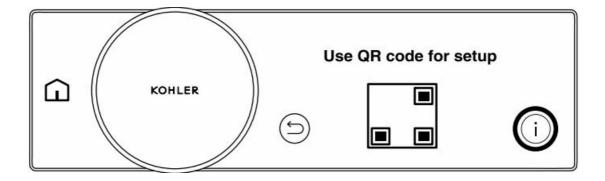
**NOTE:** If your device does not have the ability to scan a QR code, press the "i" icon to view the Anthem+ System Controller webpage address and proceed to the next section.
