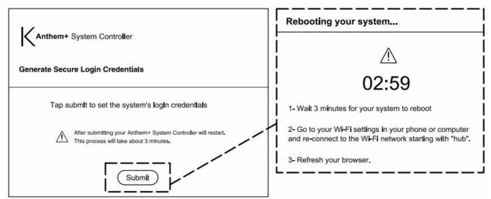
**NOTE:** If you connected to the Anthem+ System Controller webpage using the QR code, proceed to the "Enter Unique PIN" section.
