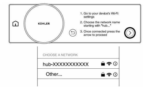
**NOTE:** The system controller is now in access point mode and discoverable by your device's Wi-Fi settings. If no action is taken for 30 minutes, the system controller will no longer be in access point mode. Press the back button and then press the arrow to return the system controller to access point mode.
