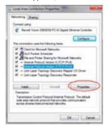
3. Setting IP address manually: Type IP address is 192.168.10.x (x is from 2 to 254), and Subnet mask is 255.255.255.0. Type the Router's LAN IP address (the default IP is 192.168.10.1) into the Default gateway field.
