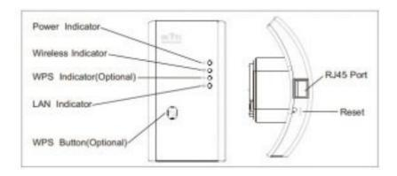
**NOTE:** If you need to the Wi-Fi Repeater, you need press and hold the reset button inside the tiny hole for seconds.
