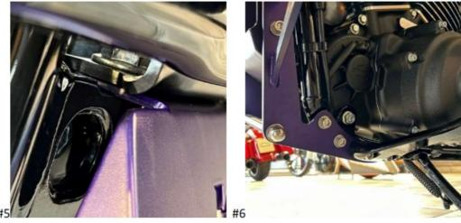
7. Place the Kodlin Engine Guards left and right sides between the frame and foot controls. See pictures #6 and #7 below.
