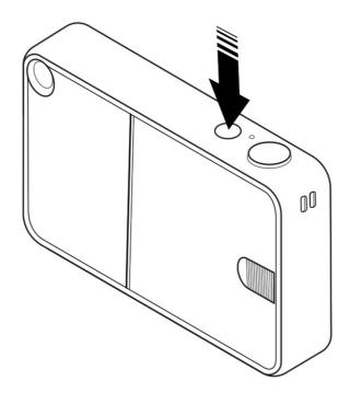
Press the power button for 3 seconds to turn on the camera.
