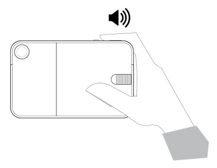
When you're ready to take a photo, press down on the shutter button and hold the camera still until you hear an alert.
