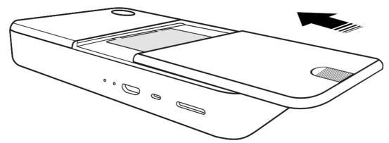
Slide the camera door back onto the camera.
