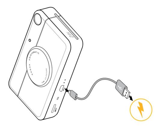
Charge the camera with a USB cable before use.
