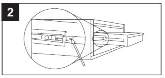
2. Pull the release lever up on the left side of the drawer. Holding both levers, pull the drawer out until the drawer releases from the drawer slides.
