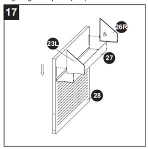
18. Secure the left and right storage cage side panels (23L and 26R) with screws (AA and BB).
