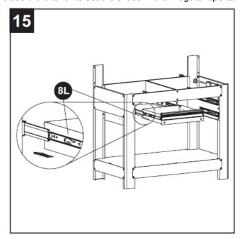
**Note:** The drawer will stop initially at the detent on the drawer slide. Apply even pressure against the front of the drawer to engage the detent. Do not slam the drawer shut.
