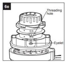
• Insert the new line into the eyelet. Feed the line until the end of the line comes out of the other side eyelet of the spool base (Fig. 6f).
