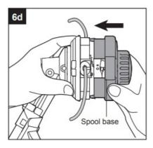
**NOTICE:** Make sure that the tabs on the spool base snap into place, otherwise the spool will come out during operation.
