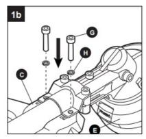
• Use the supplied hex key to secure the guard in place with the washers and bolts.
