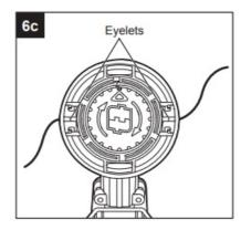
Align the two tabs on the spool base with the slots on trimmer head and press it until it snaps into place (Fig. 6d).
