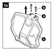
• Lift the trimmer head (E) and face it downward; align the two mounting holes in the guard with the two assembly holes in the base of the shaft. Make sure that the inner surface of the guard faces toward the trimmer head (Fig. 1b).
