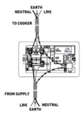
These products have no cable entry and should only be used for "hard wired" installations.
