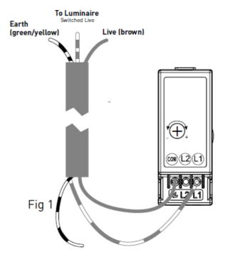
For a multiple gang dimmer please repeat the wiring method for each dimmer.
